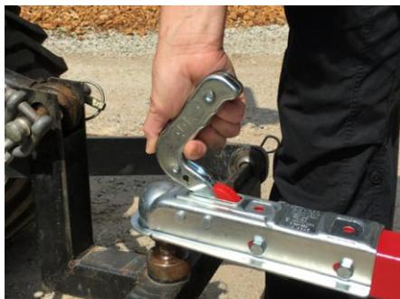
Holding latch in lift the handle to uncouple from the tow ball.
