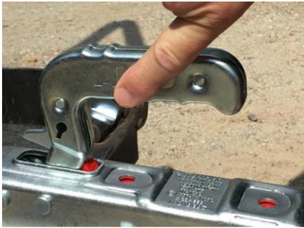
To release the hitch handle, press the indicated latch.
