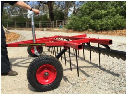
Once the surfaced has been groomed, wind the arena rake up using the jack lift to transport the rake from the arena. Keep winding until you hear a series of clicks, indicating maximum height is achieved.
