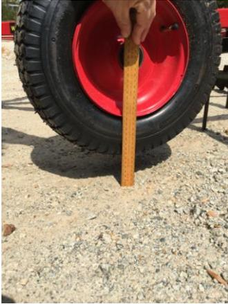
After transporting the arena rake to the arena, using the lift jack lower the arena rake to the arena surface this is achieved by raising the wheels off the surface of the arena. Raising the wheels will also lower the tines (this is one action). Therefore you need to raise the wheels to the depth you require the tines to penetrate the top surface of your arena. For example, raising the wheels 5cm from the surface will allow the tines to penetrate the top surface 5cm.
