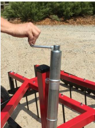
This is the lift jack, which will raise and lower the arena rake for transporting.
