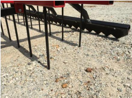
The tines and the grooming blade are preset and should not require adjustment. The tips of the tines and the grooming blade should touch the surface at the same time. The long black blade at the back is called the grooming blade, this controls the depth of the tines.
